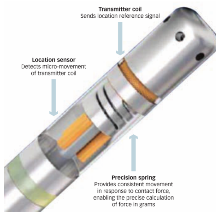
Figure 1.6: THERMOCOOL® SMARTTOUCH™ catheter [37].
