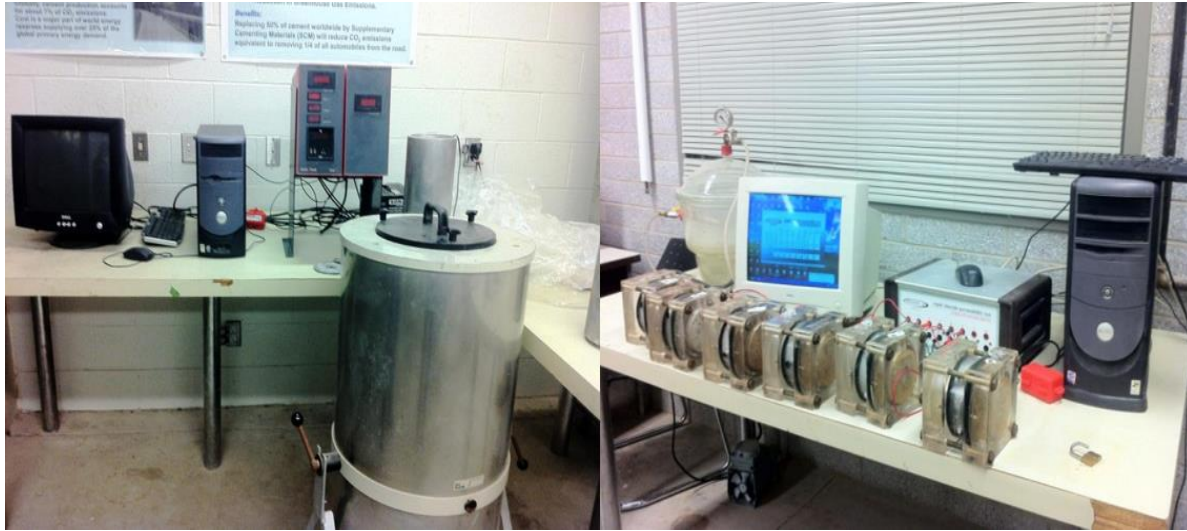
Figure 2: Test setup for heat of hydration (left) and rapid chloride permeability test (right)
