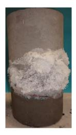
Figure 1: Salt crystals on concrete surface
