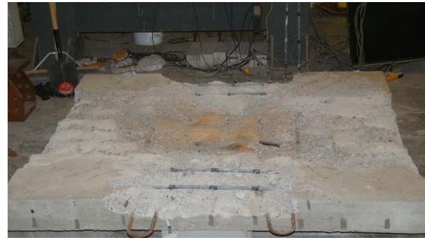
Figure 13: Delamination area around the corroded region
