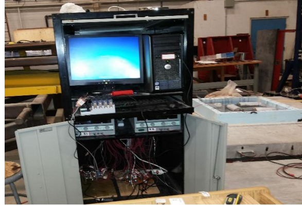
Figure 3: Corrosion current monitoring by data-acquisition system
