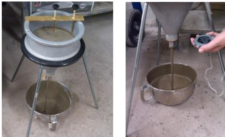
Figure 1: Grout flowability measurement using flow cone method.
