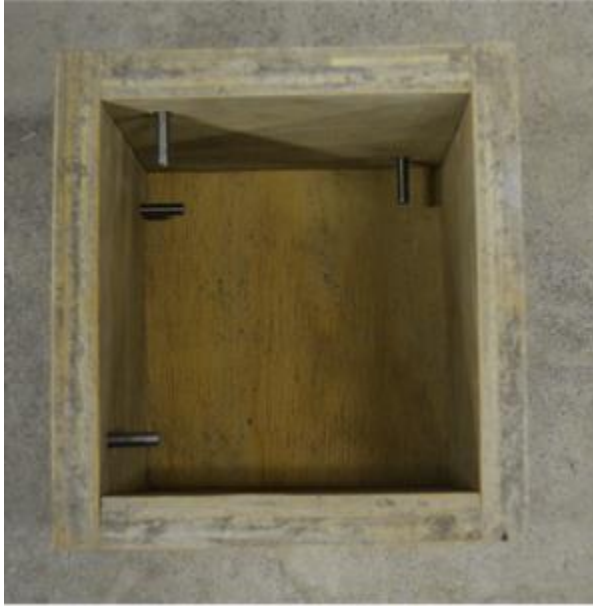
Figure 1: Moulds for cubes
