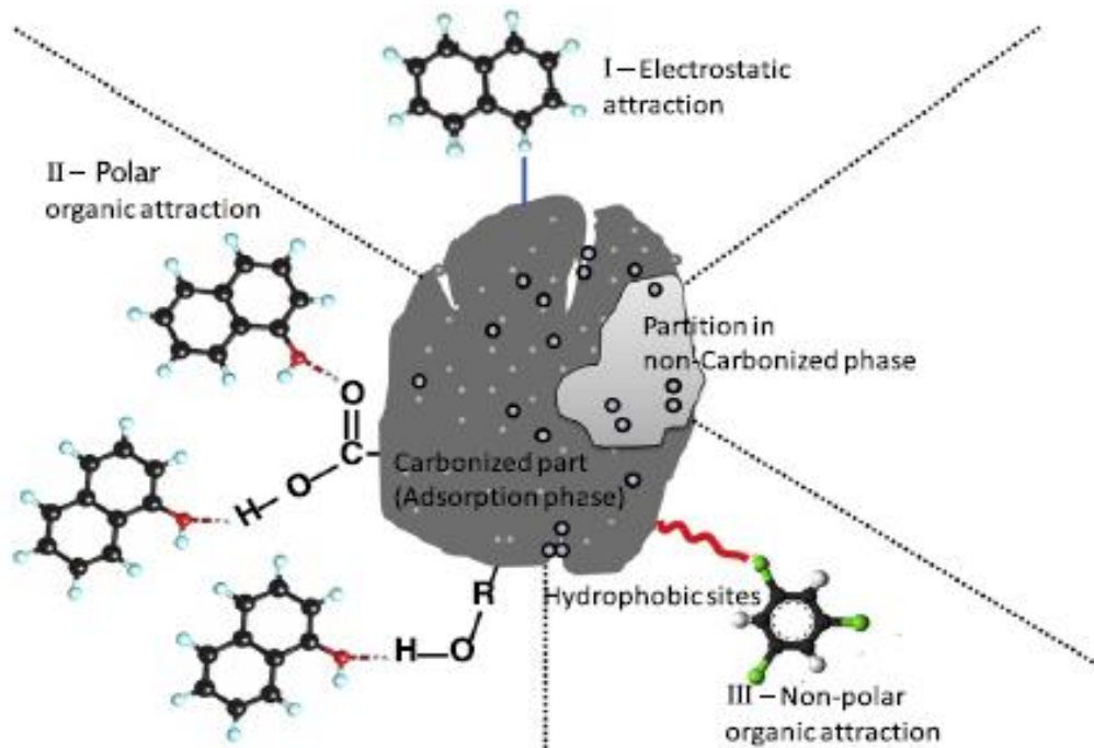
Figure 5.2. Probable mechanisms of the interactions of organic contaminants with biochar (Ahmad, M. et al., 2013)
