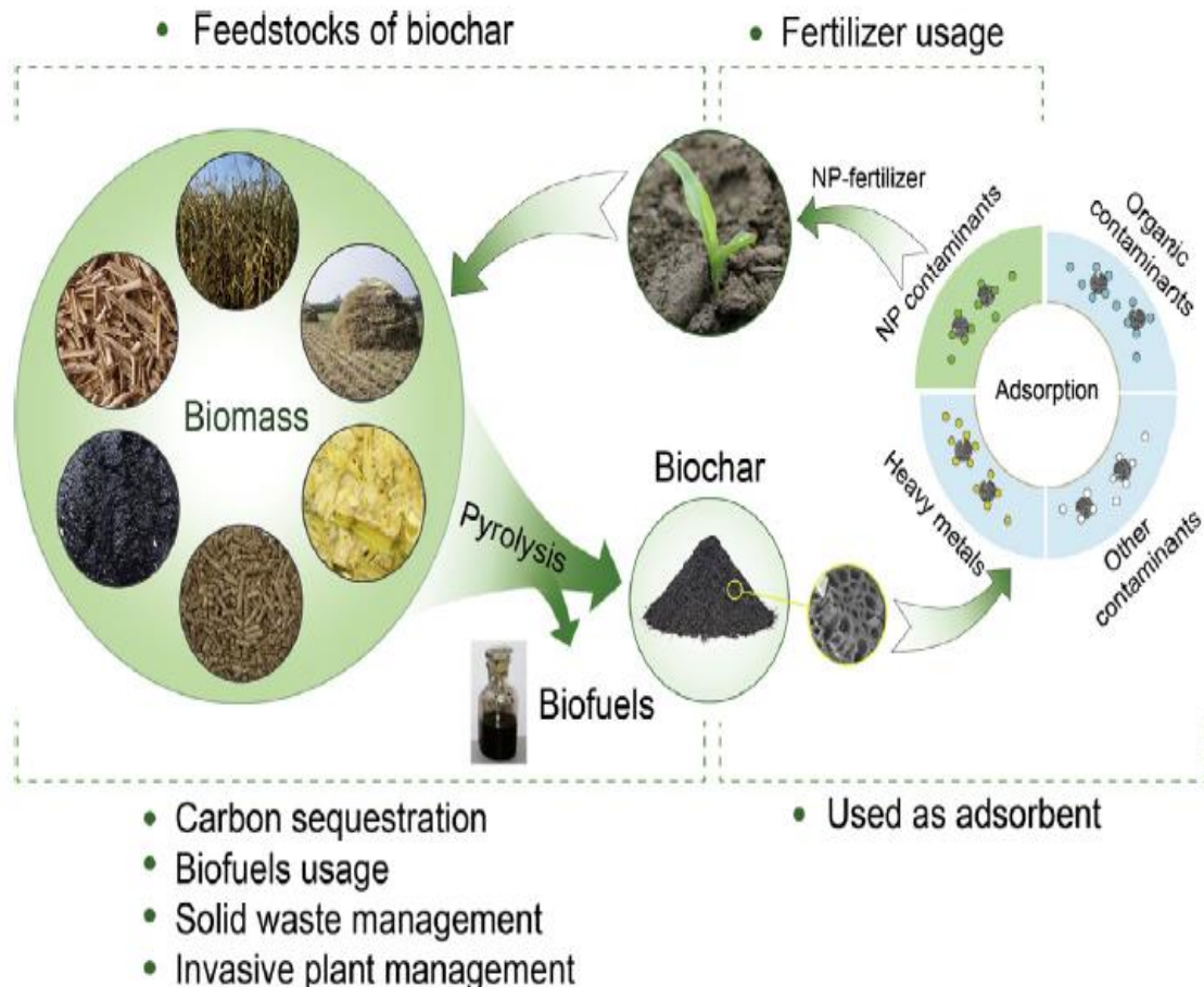
Figure 0.4. Production and application of biochar for wastewater treatment as an effective adsorbent (Tan, X. et al., 2015).
