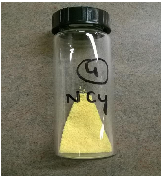
Figure 4.5. Yellow \text{In}_2\text{O}_3 nanocrystals obtained after calcination at 400^\circ\text{C} for 2h.
