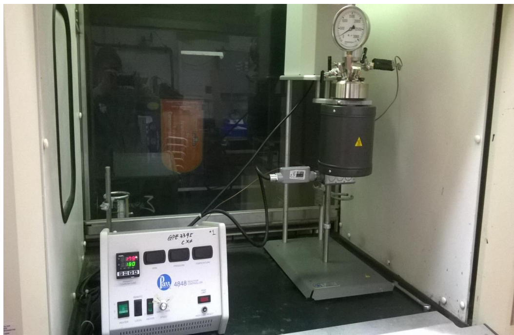
Figure 4.1. Stainless steel autoclave used to synthesize nanocubes, nanoplates and porous microspheres in Parr reactor at 180^\circ\text{C} \pm 2^\circ\text{C} for 16h
