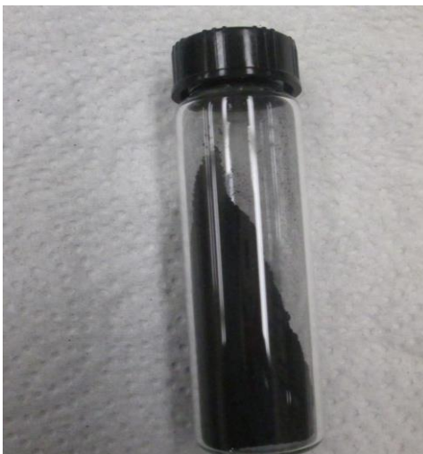
Figure 5.6. Biochar obtained after slow pyrolysis at 700°C with a ramp temperature of 7°C/min for 1h.
