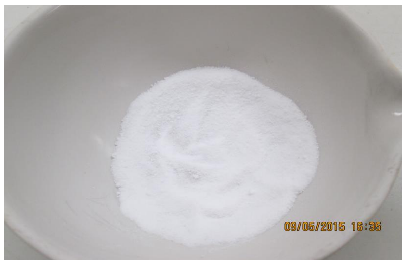
Figure 4.4. White precipitate of \text{In}(\text{NO}_3)_3 \cdot 4.5\text{H}_2\text{O} after co-precipitation followed by drying at 80^\circ\text{C} for 24h.
