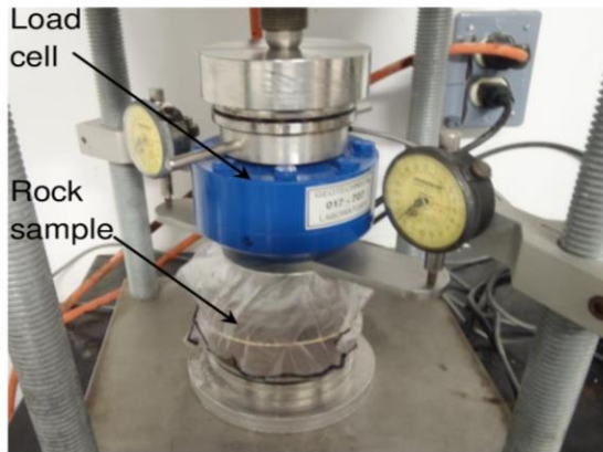
e) null swell test (experiment)
