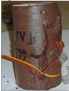
Figure 4.10. Triaxial compressive strength test performed on: (a) intact specimens and specimens soaked for hundred days in: (b) water; (c) polymer solution and (d) bentonite solution; (1) vertical specimens, (2) horizontal specimen.
