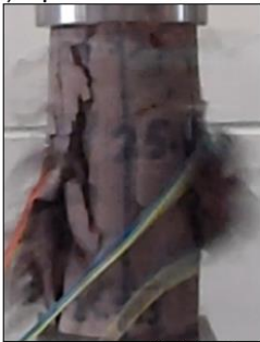
Figure 4.9. Unconfined compressive strength test performed on: (a) intact specimens and specimens soaked for hundred days in: (b) water; (c) polymer solution and (d) bentonite solution; 1) vertical specimens, 2) horizontal specimen.
