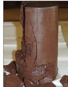
Figure 4.10. Triaxial compressive strength test performed on: (a) intact specimens and specimens soaked for hundred days in: (b) water; (c) polymer solution and (d) bentonite solution; (1) vertical specimens, (2) horizontal specimen.
