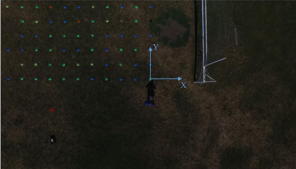
Figure 15. The measurement grid that was used to measure camera error. The distance between each cone is 1m. The X-Y coordinate system was set up at the focal point of the camera.
