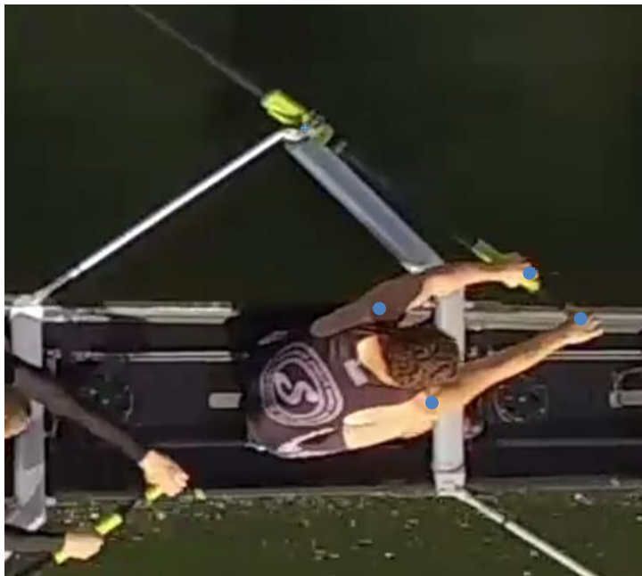
Figure 12. An image of an individual rower taken by the drone with the tracked points marked in blue.
