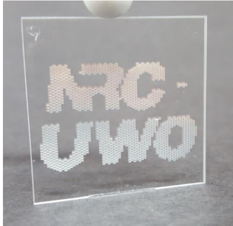
Figure 5.9 Fabricated logo comprised of RTP structures
