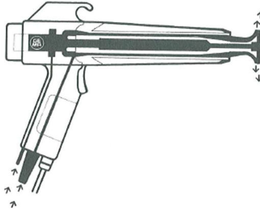
Figure 2.13 Tribo charging gun (source: Ransbwg Gema AG)
