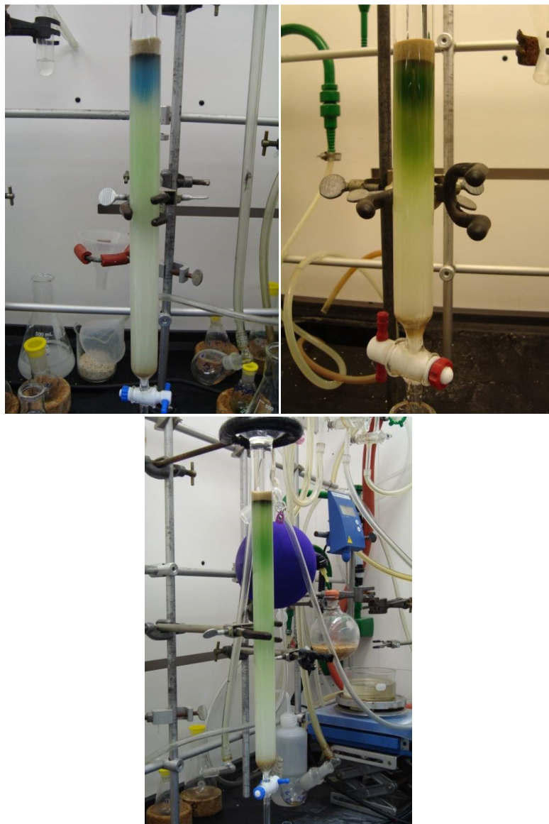
Figure 17. The varying bands of decomposed cobalt catalyst (modp and piper ligands).
