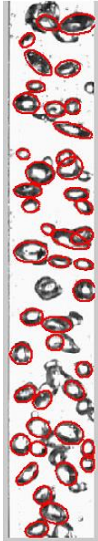
Figure 2.5: The identified bubbles approximated as ellipses are shown plotted over an original image.
