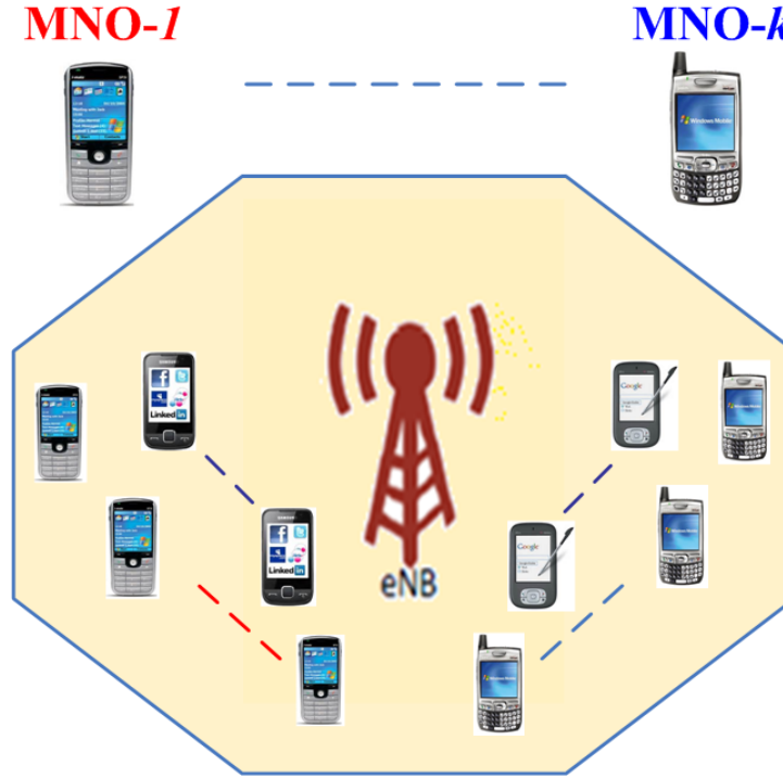
Figure 3.1: MNOs sharing radio RBs in a single eNB.
