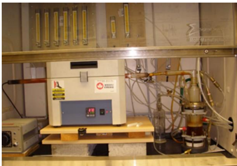
Figure 2.1 A picture of Aerosol-Assisted Chemical Vapour Deposition.
