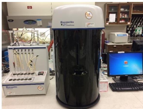
Figure 2.6 A picture of TriStar II Plus Analyzer.
