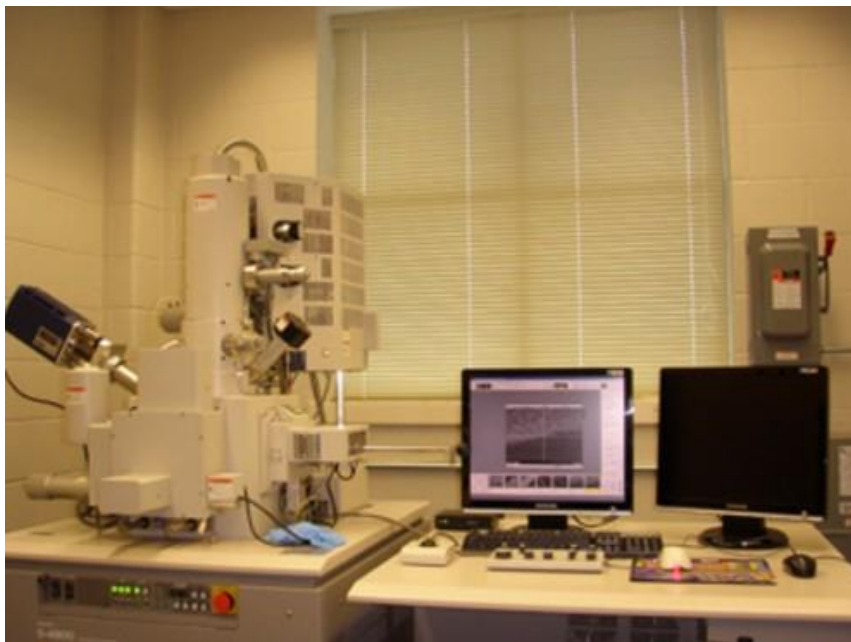
Figure 2.2 A picture of Hitachi S-4800 high-resolution scanning electron microscope.
