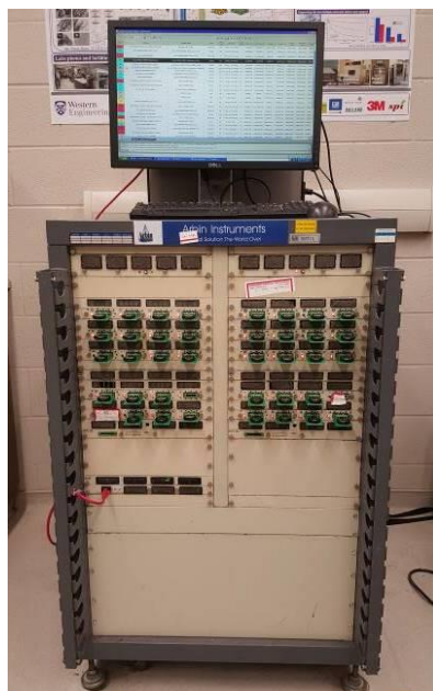
Figure 2.10. Photo of the Arbin Instruments BT-2000 battery testing system.
