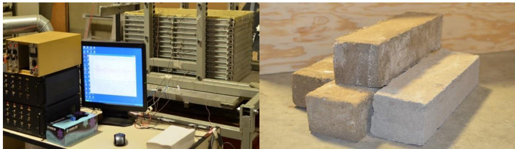
Figure 3-2: Test setup including (from left to right): data acquisition system, the electric control module, shaking table with the mounted flexible container with 12 frames; and sand-cement blocks representing frozen soils.
