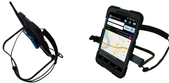
Figure 2: Portable Bluetooth and Wi-Fi scanner device use in the study
