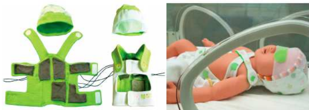
Figure 1-2 A prototype of the smart jacket (left) and a baby mannequin wearing the smart jacket inside the incubator (right). (Copy from [12])
