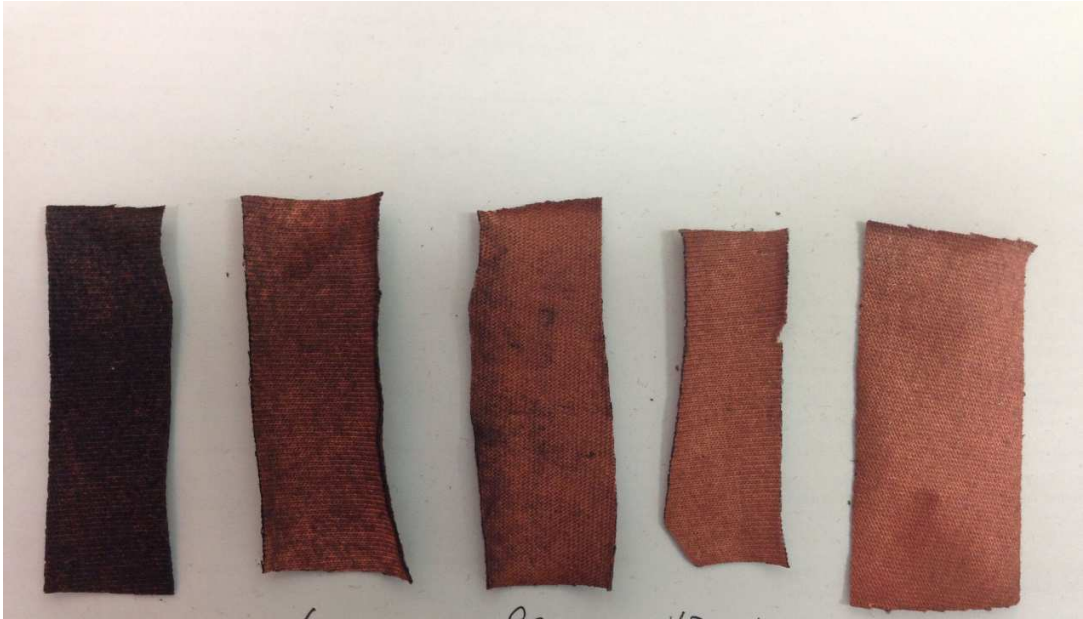
Figure 2-14 From left to right, color of each cotton fabric sample at different ELD plating time 30 , 60, 90, 120 and 150 min.
