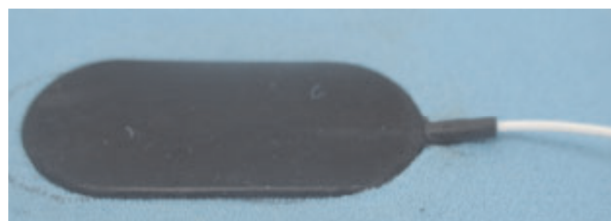
Figure 1-20 Dry electrode made of conductive rubber and integrated into a garment with shielded cable. (Copy from [39])
