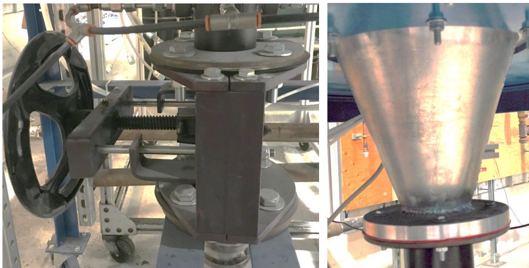
Figure 2-3. Left: Pinch valve. Right: Cone frustum section
