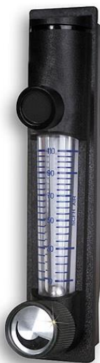
Figure 2-11. Flowmeter employed in the experiments (FI-807-V)
