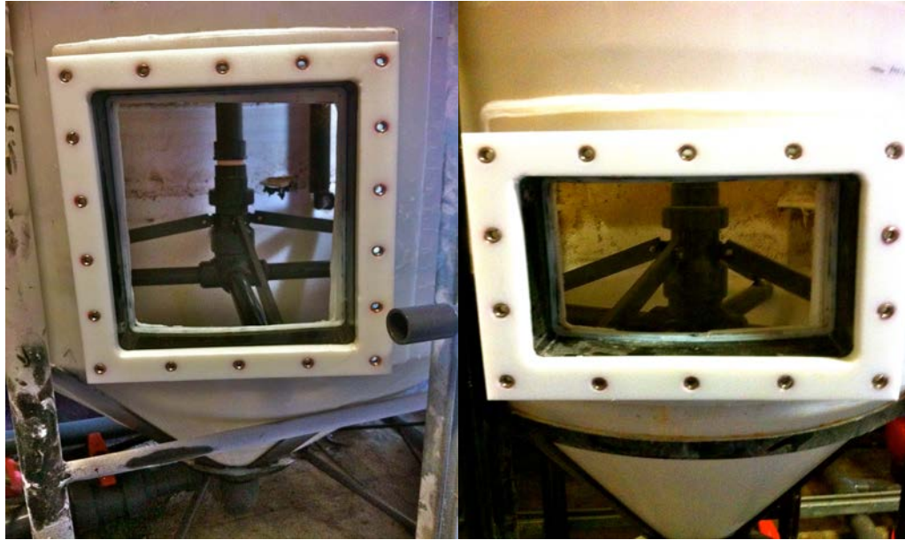
Figure 3.6: Fluidization Window Installation on Mobile CFBBR Unit. (Aerobic on the left, Anoxic on the right)
