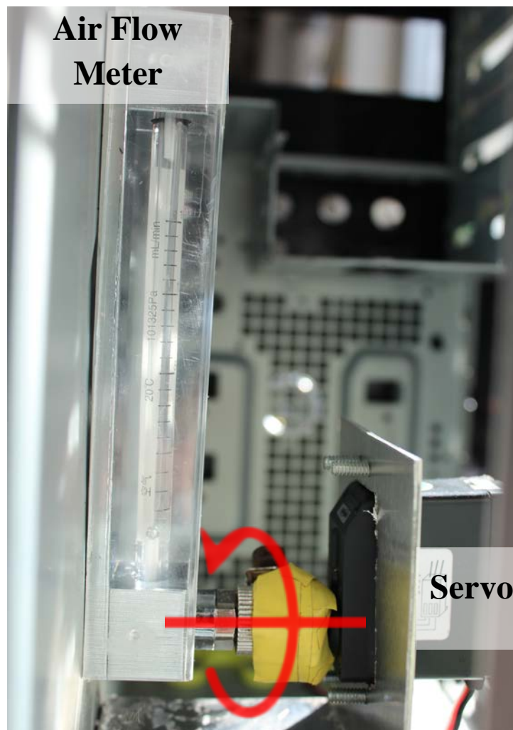
Figure 4.12: Servo Attached to Air Flow Meter to Control Air Supplied to PNFBR
