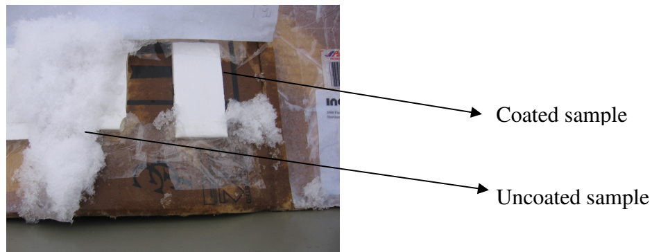
Figure 50-21: The snow test of coated and uncoated samples
