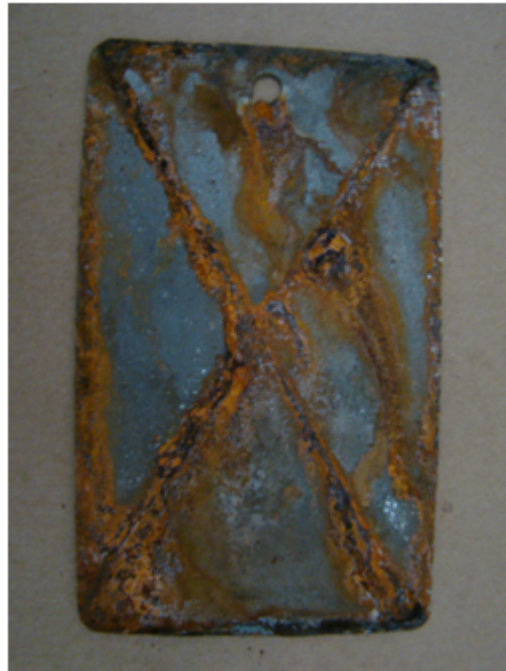
Figure 06-5: The sample coated with polyurethane conductive coatings without nanoclay after 500 hours salt spray test
