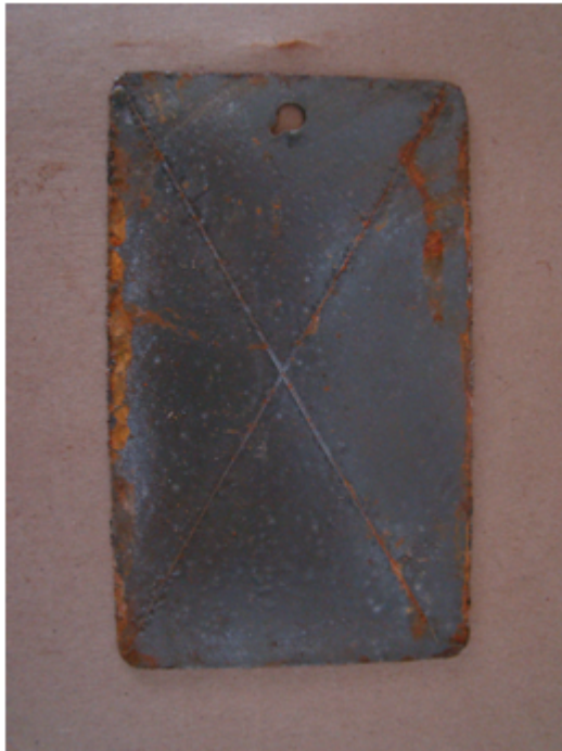
Figure 06-7: The sample coated with nano clay (5 \mu\text{m} ) polyurethane conductive coatings after 500 hours salt spray test
