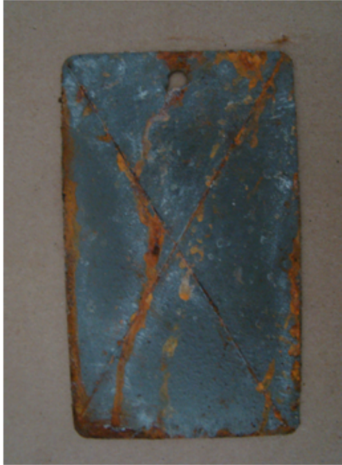
Figure 06-6: The sample coated with nano clay (25 \mu\text{m} ) polyurethane conductive coatings after 500 hours salt spray test
