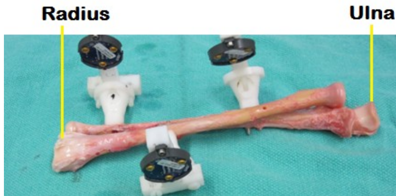
Figure 2.6 The radius and ulna, denuded of soft tissue with mounted infrared optical marker triads © Braden Gammon.
