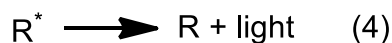
Figure 14 General mechanism for annihilation ECL, where radical cation and radical anion to form R^* . This excited species relaxes back down to the ground state and releases light.
