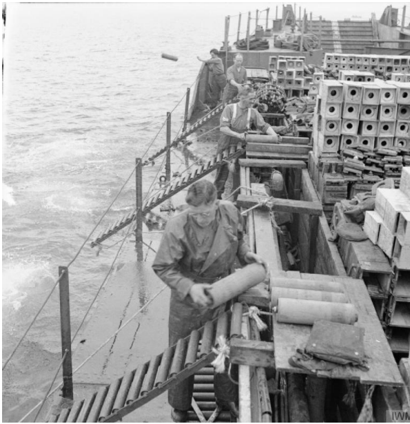
Photo 20 On arrival at the ammunition dumping ground off Cairnryan, members of the Royal Army Ordnance Corps (RAOC) place shells on gravity rollers that take the ammunition over the side of the ship and into the sea. Note the man in the background who is simply throwing ammunition overboard. © IWM (H 42208)
