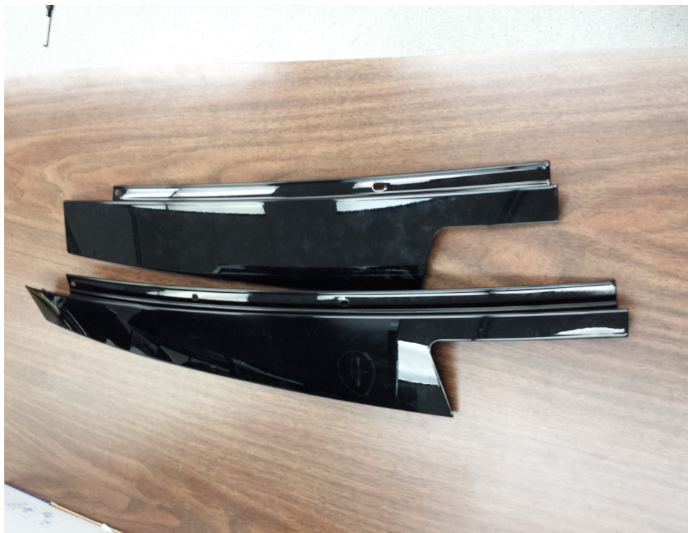
Figure 4.2: Window pillars comparing the longer and shorter window pillars for front and back placement
