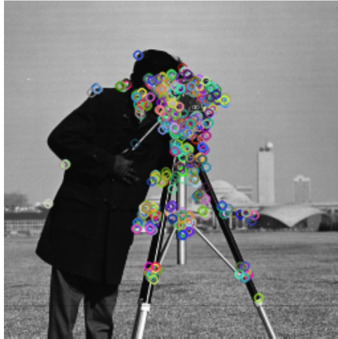
Figure 2.2: ORB features found in an image
