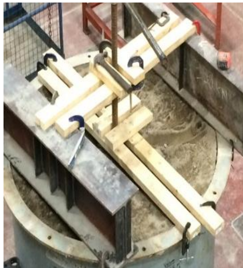
Figure 4.3: Guiding system to insure verticality of hollow bar micropiles
