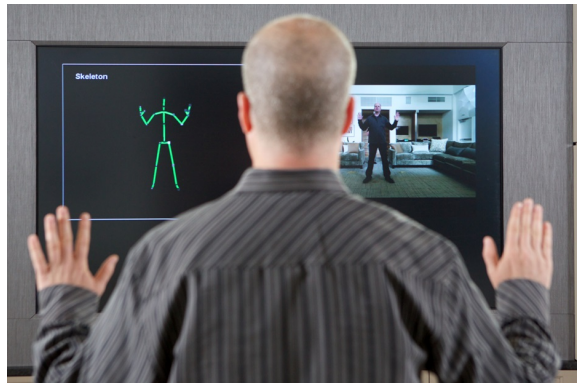
Figure 1.18: Microsoft XBox Kinetic used for mapping the human skeletal model to the user in the frame of reference [42]
