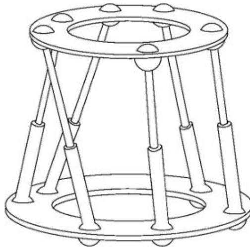
Figure 1.23: A Stewart platform for simulating 6DOF passive wrist motion uses six actuators to achieve 3 degrees of freedom of translation and rotation each with the wrist mounted on the top surface of the platform [57]
