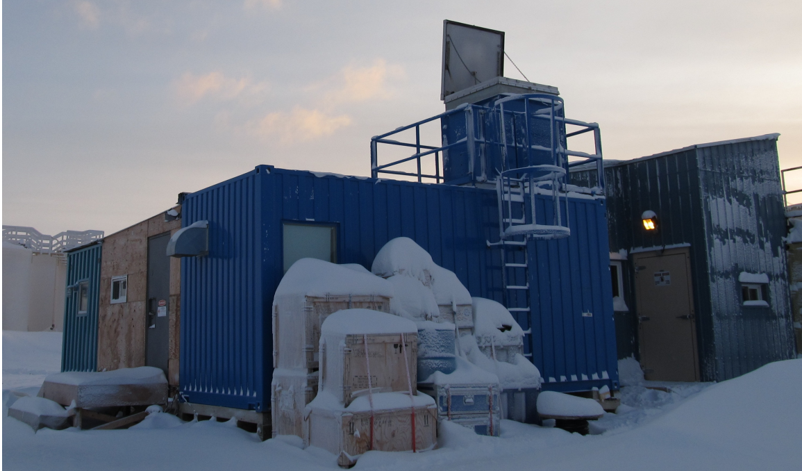
Figure 3.2: CRL lidar container with roof hatch open
