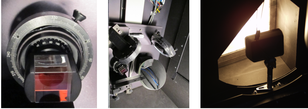
Figure 8.2: The extra polarizer is a linearly polarizing cubic prism. It is placed immediately downstream of the focus stage and is rotated by hand. The glassine sheet ensures that all light entering the cubic prism is unpolarized. The calibration lamp is securely bolted onto the telescope frame.
