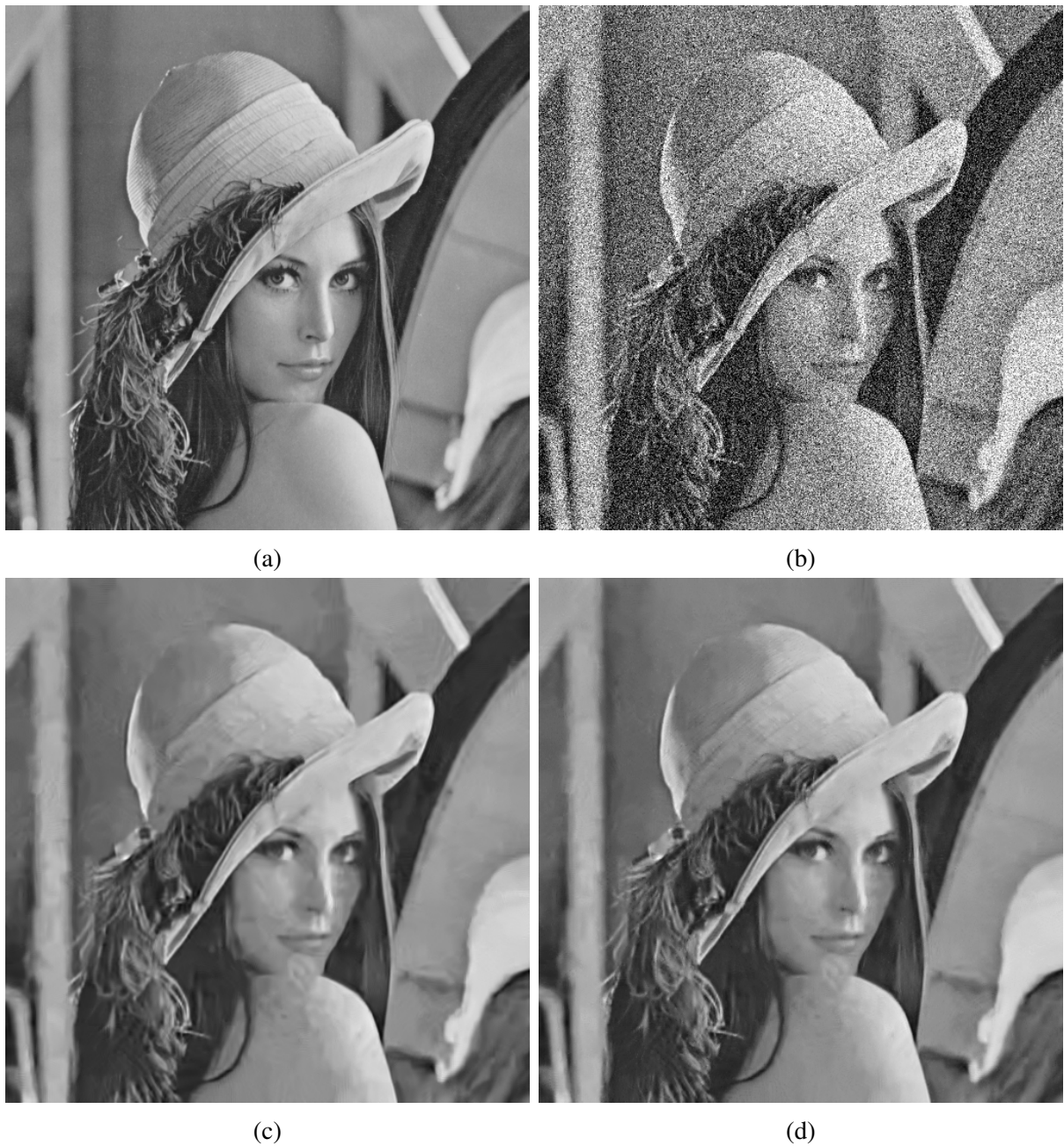
Figure 5.11: Subjective Comparison of Lena Image (a) Original Lena Image. (b) AWGN added with \sigma = 50 (c) Denoised Image using BM3D (PSNR=29.05) (d) Denoised Image using Proposed Method (PSNR=30.54)
