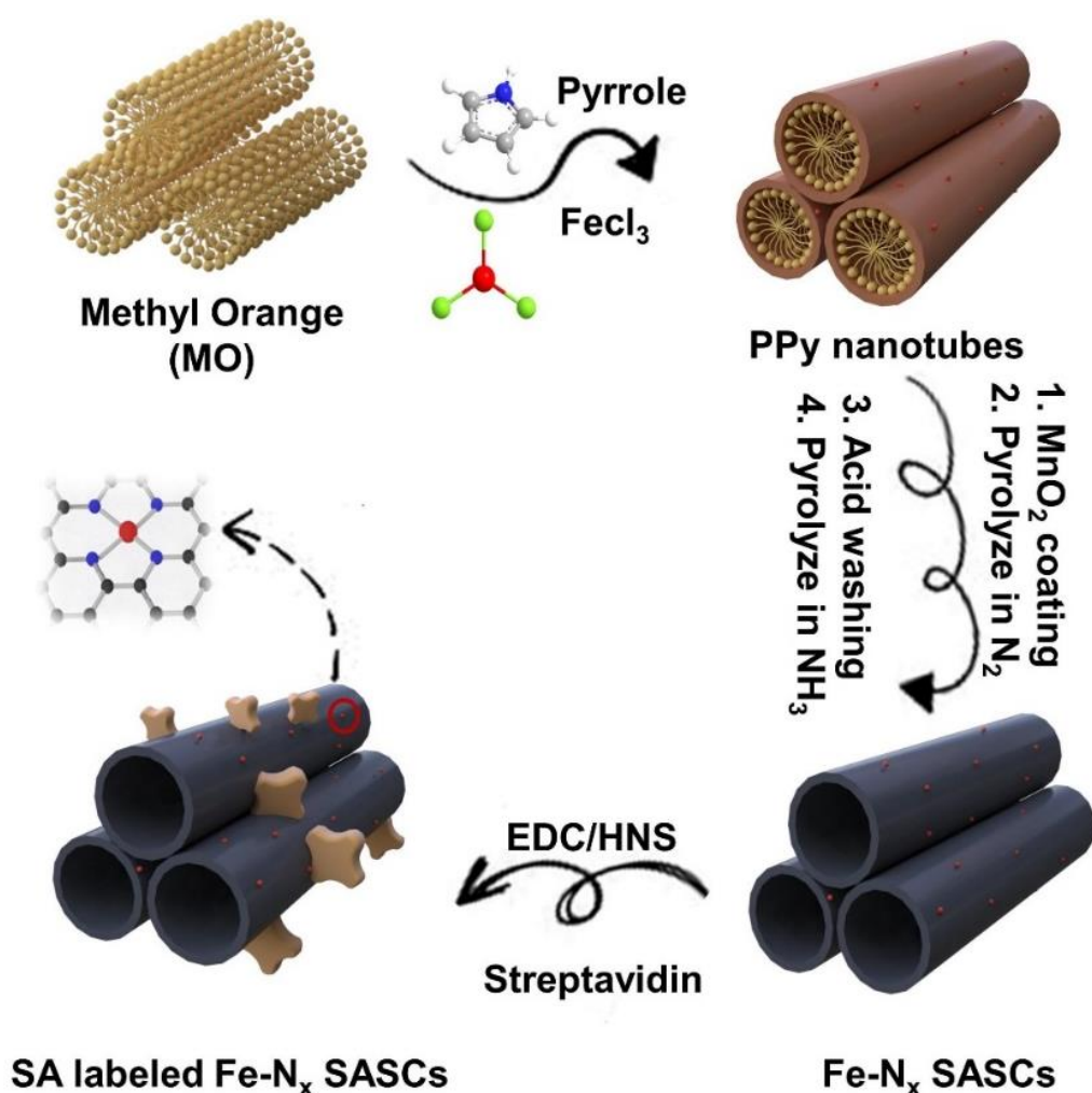
Figure 3.1 Schematic diagram of preparing SA-labeled Fe-N x SASCs.
