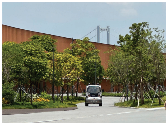
FIGURE 10. Situations where the presence of tree shade potentially impacts the perception results and navigation performance of AVs, especially when the trees sway in the wind, causing fluctuations in the boundary of the drivable area.
