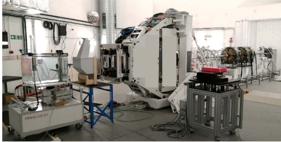
Figure 2. Photograph of Beamline A with PTW water tank and IBA LYNX detector positioned at the reference plane.
