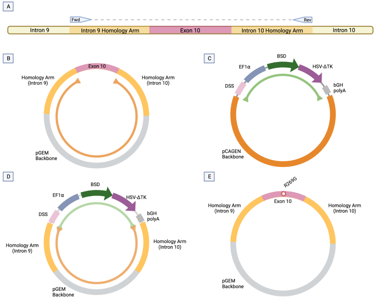
Figure 3.10: HDR Donor Template Cloning Strategy. (A) Using H9 hESC gDNA, a high-fidelity PCR reaction amplified \sim 1800 bp of uninterrupted genomic sequence encompassing the WT target site (ITPR1 Exon 10 is shown as an example). The forward and reverse primers in this reaction mark the external limits of the homology arms. (B) An intermediary plasmid was prepared by cloning the PCR product into a pGEM T-Easy vector. This was used as template in an inverse PCR reaction to generate a linear amplicon (inner orange semi-circle) containing the 5' homology arm (ITPR1 Intron 9 shown), the pGEM backbone, and the 3' homology arm (ITPR1 Intron 10 shown). This amplicon is ligated into the CIRCES cassette-containing amplicon, which was similarly PCR amplified (green inner semi-circle) from (C), the pCAGEN vector containing the assembled cassette. (D) The ligated amplicons form the first HDR Donor plasmid, which is used in the Insertion Stage. It is important to note that a small region encompassing the target site (here ITPR1 Exon 10, shown in red) is deliberately excluded from the first HDR template. This feature prevents Cas9 re-cutting after correct insertion. (E) The second HDR Donor plasmid, to be used in the Replacement Stage, contains the desired mutation to be introduced (ITPR1 Exon 10 mutation R269G shown as an example) and the immediately adjacent target context (here ITPR1 Exon 10, shown in red) that is not present in the first HDR donor plasmid. This replacement stage HDR donor template is cloned by simple site-directed mutagenesis to the intermediary wild-type pGEM plasmid (B).
