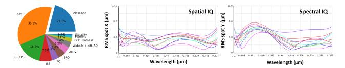
Figure 10: Breakdown of the overall image quality budget by subsystem, which is quite similar at all wavelengths. The contribution from the VLT itself is highlighted for reference. The dominant contribution comes from the BlueMUSE spectrograph, and we show in the right panels the rms spot radius of the spectrograph in both directions (spatial and spectral).
