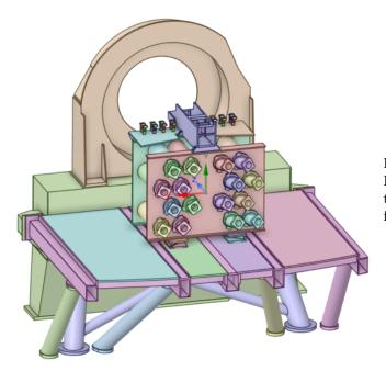
Figure 3: General idea of the mechanical structure of BlueMUSE on the VLT Nasmyth platform, including the 16 IFUs standing out at the back as well as the fore-optics in blue at the top.
