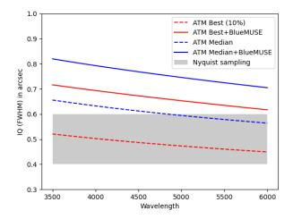
Figure 9: Global image quality (FWHM of the PSF) expected for BlueMUSE observations as a function of wavelengths, under two cases of atmospheric turbulence (10% best and median seeing conditions). When adding the contributions from the telescope and instrument we can see that the PSF will always be at least Nyquist sampled by the  $0.2^{\circ} \times 0.3^{\circ}$  rectangular spaxels (grey rectangle).
