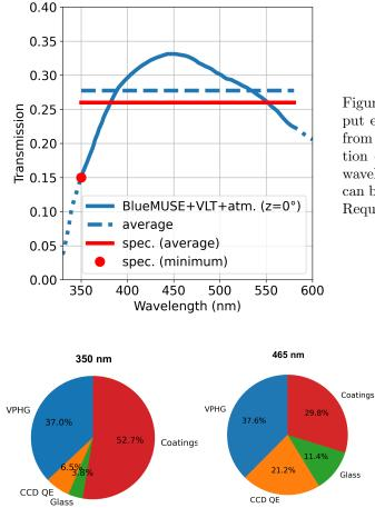
Figure 7: The blue curve shows the end-to-end throughput expected from BlueMUSE, including the contribution from the VLT and the atmosphere at zenith, as a function of wavelength. The average value over the common wavelength range is shown as a dashed line. These values can be compared with the minimum and average Top Level Requirements presented in Sect. 2 and shown in red.
