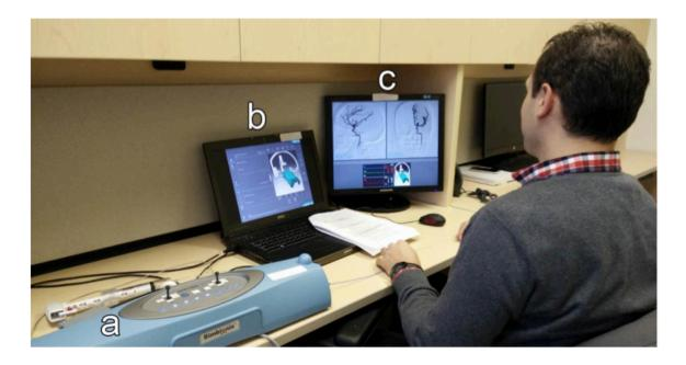
Figure 6: A participant completes a practice scenario using the simulation console (A), main patient screen (B), fluoroscopy screen (C), and pedals (not pictured).
