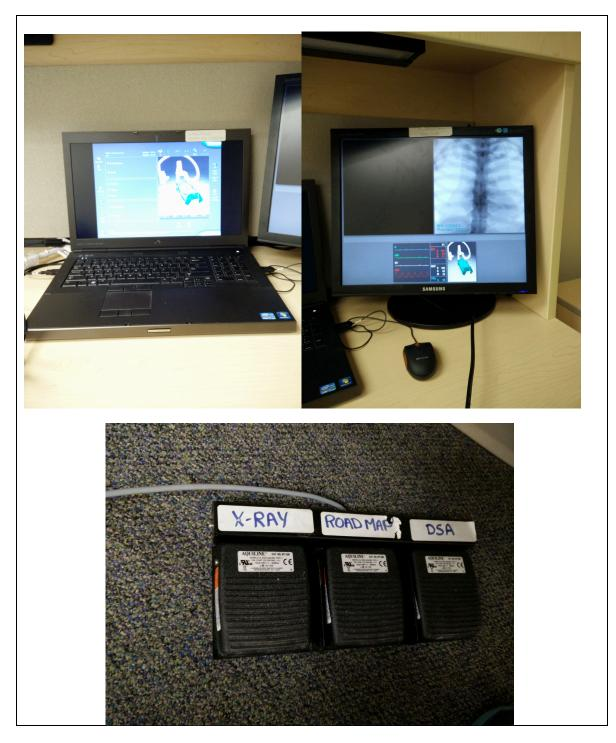
Figure 5: Computer with main display (left) and fluoroscopic monitor (right) and pedals for fluoroscopy, roadmaps and DSA (bottom)
