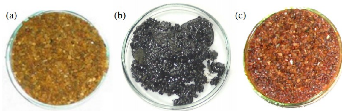
Figure 2.7: Coarse grain sand (a) without coal tar, (b) with coal tar, (c) after STAR remediation (Pironi et al., 2009).
