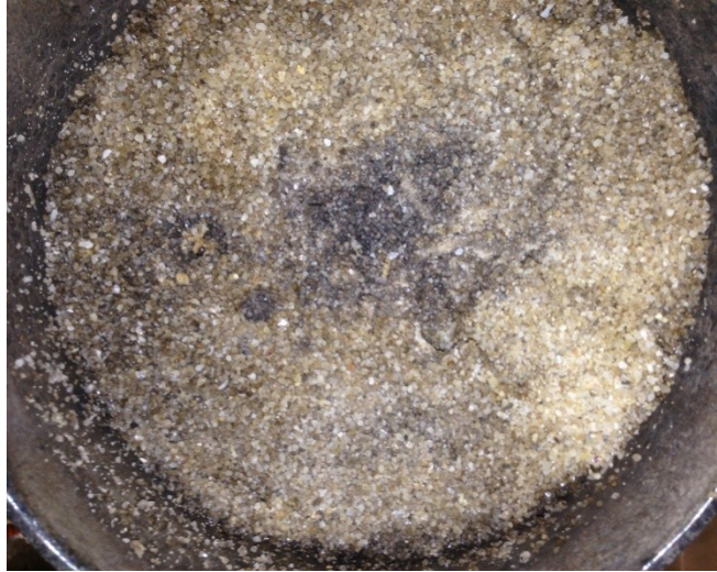
Figure F4: Example picture of the top, initially clean sand cap with condensed pyrolysate following full combustion in Experiment No. 29.
