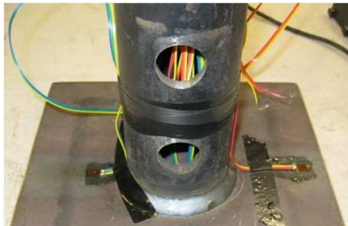
Figure B- 6 Strain gauge installation on a pile cap used for compression loading test
