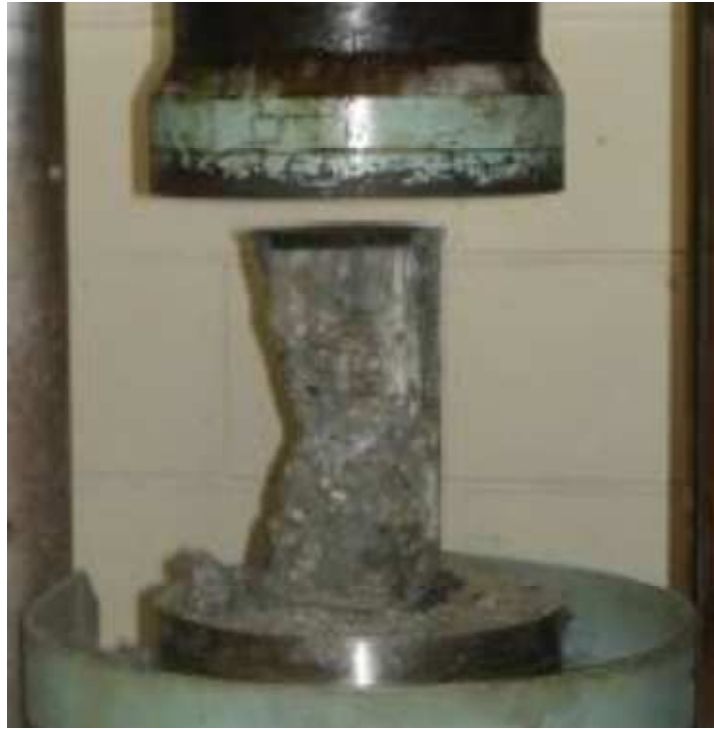
Figure A- 2 The typical observed concrete cylinder failure under compression testing
