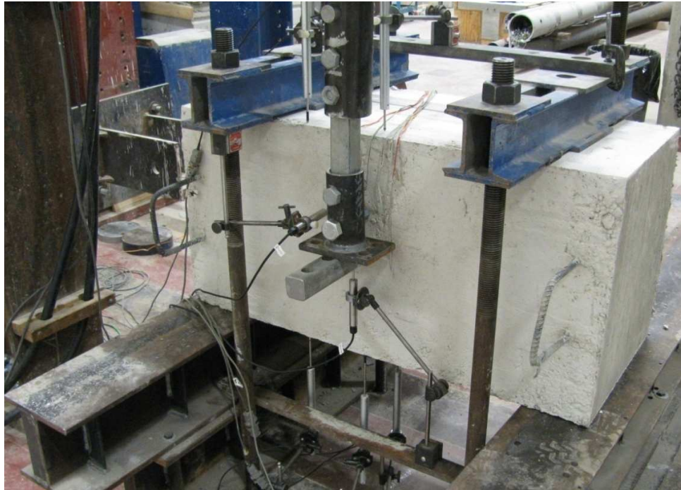
Figure 9-3 Test rig and locations of displacement transducers: a) schematic; b) actual setup
