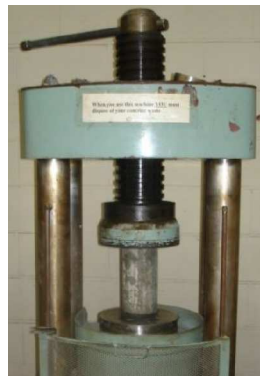
Figure A- 1 The conducted concrete compression test according to ASTM C39 / C39M
