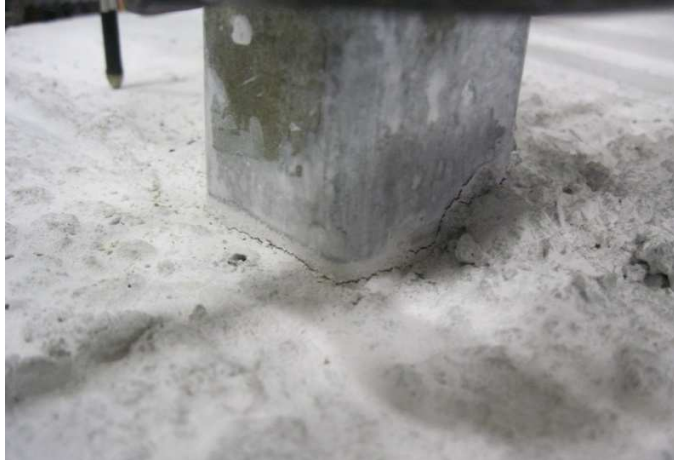
Figure 3- 5 Bond failure between the pile shaft and the surrounding concrete
