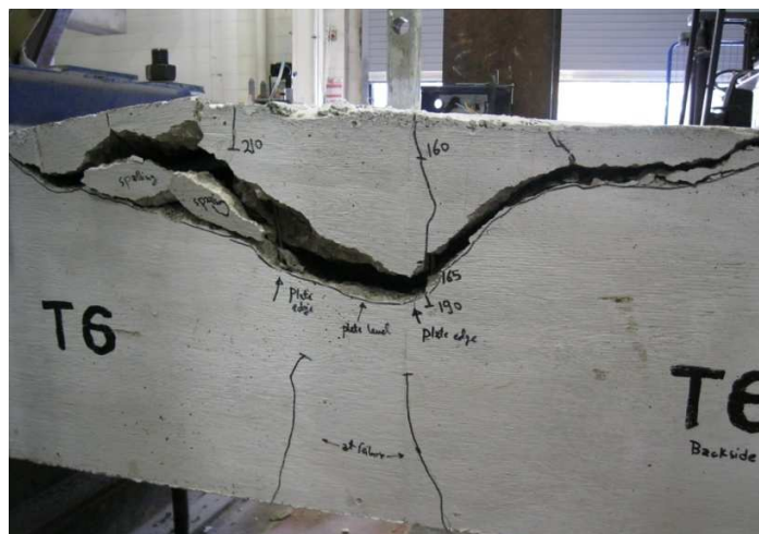
Figure 3- 12 Vertical cracks initiation after the stirrups failure on the other side of the beam
