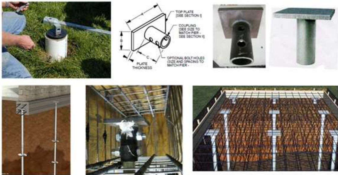
Figure 1- 2 The commonly used pile cap (i.e. New construction bracket) and its application in different types of the new reinforced concrete foundations (Perko, H. A. , 2009).
