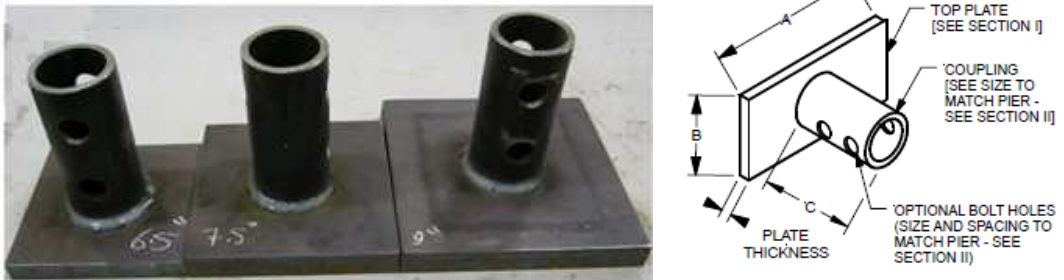
Figure 9- 1 Commonly used pile cap (i.e. New construction bracket )
