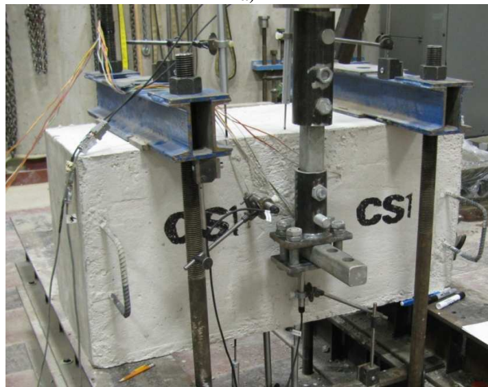
Figure 9- 5 Test rig and location of displacement transducers for cyclic shear loading: a) schematic; b) actual setup
