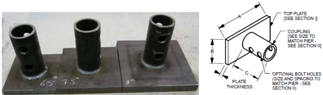
Figure 6- 1 Commonly used pile cap (i.e. New construction bracket)
