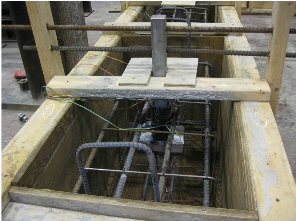
Figure B- 2 The used pile fixation system
