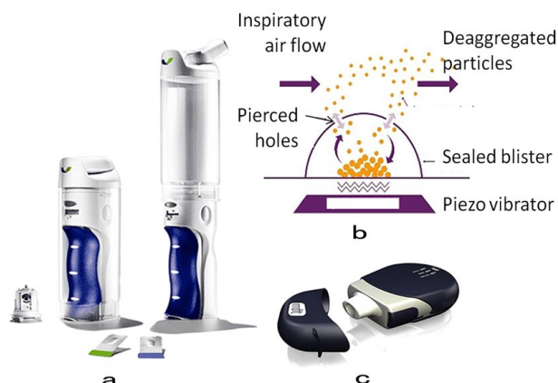
Figure 2.3: Active dry powder inhalers. a, Exubera®; b, principle of Microdose® device; c, Microdose® device
