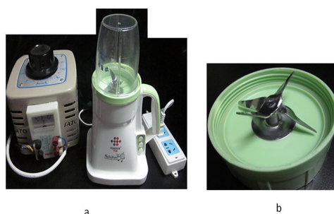
Figure 3.24: Pictures of the high shear mixer. a, a voltage transformer and the mixer; b, the altered blades.
