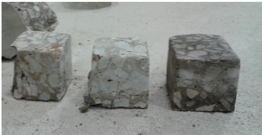
Fig. 2.2: 50 mm cubes for compressive strength test.
