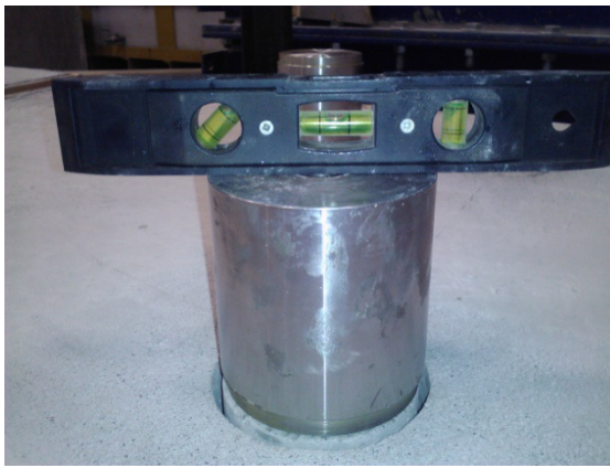
(a) Bonding of the steel disk using epoxy.
