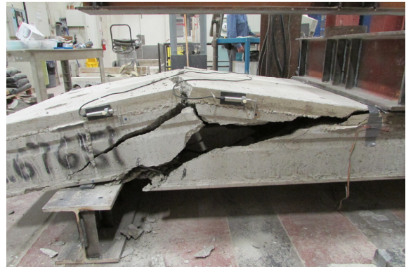
(f) FRA2-3 (flexure-shear failure).
