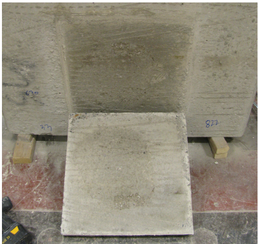
(a) Interface shear failure
