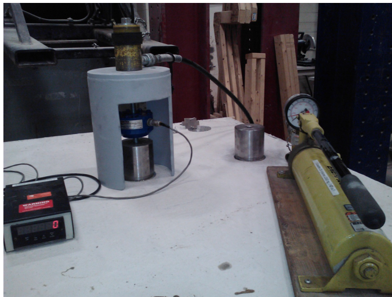
Fig. 2.7: Pull-off apparatus (dimensions in mm).
