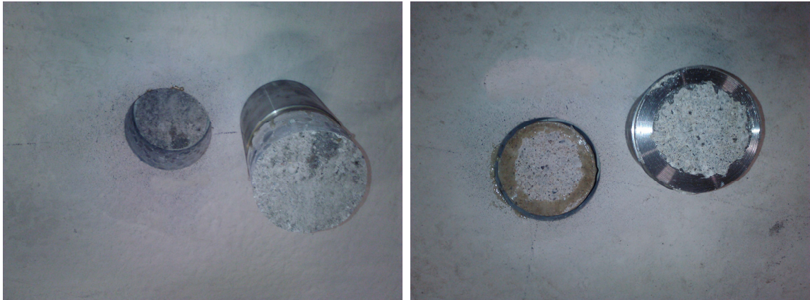
(a) Interface failure (I)
