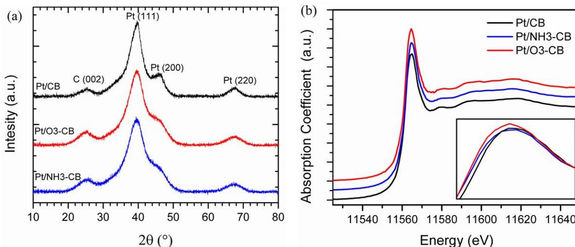
**Figure 4-4.** XRD (a) and XANES (b) and spectra of Pt/CB (black), Pt/O3-CB (red), and Pt/NH3-CB (blue). The inset is (b) is a highlight of the XANES absorption edge at 11565 eV.
