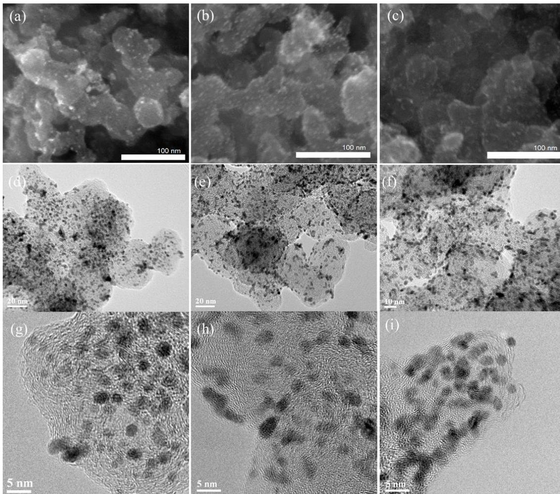
**Figure 4-3. SEM, TEM, and high-resolution TEM images of Pt/CB (a, d, g) Pt/O3-CB (b, e, h) and Pt/NH3-CB (c, f, i) showing good distribution of particles and relatively homogeneous particle size.**
