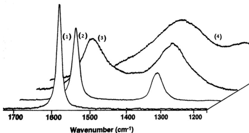
**Figure 2-7. (a) Raman spectra for (1) highly ordered graphite, (2) polycrystalline graphite, (3) amorphous carbon, (4) diamond-like carbon [14]. The D- and G-bands at 1350 and 1590  $\text{cm}^{-1}$ , respectively, are noticeable especially in (2) and (3).**
