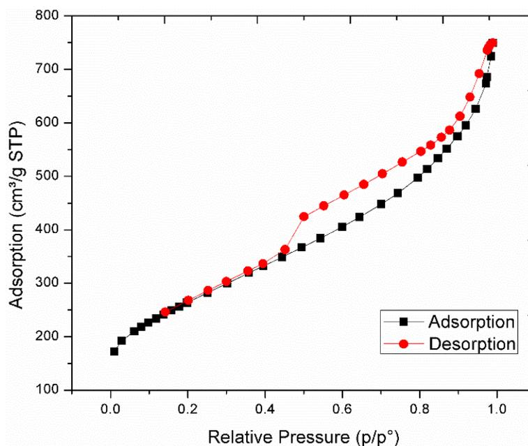
**Figure 2-5. Typical N<sub>2</sub> gas sorption isotherm of a high surface area material with adsorption points in black and desorption in red. The hysteresis during desorption is a result of micropores.**
