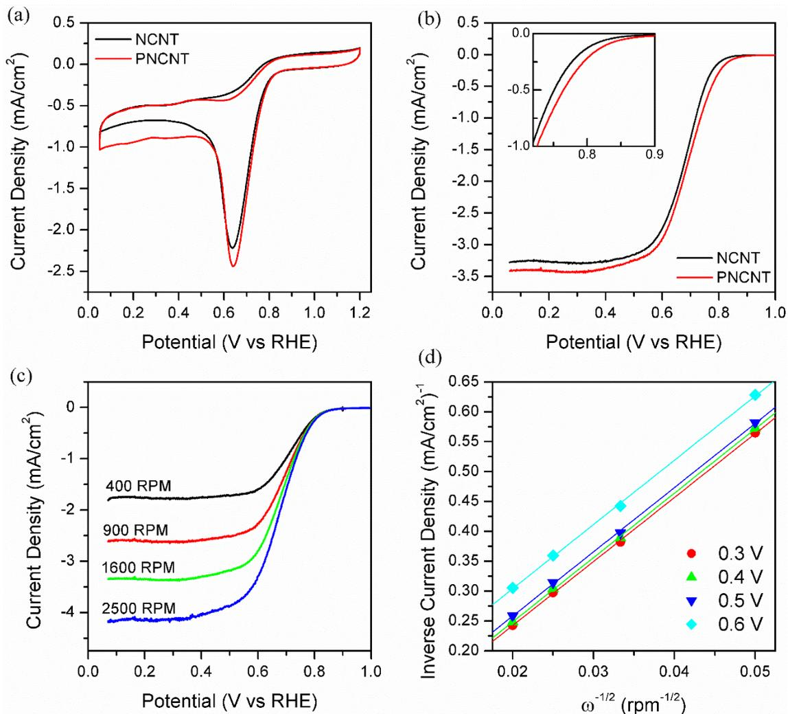
**Figure 3-6.** (a) CVs recorded in  $O_2$  saturated 0.1 M KOH solution for NCNTs and PNCNT (b) ORR polarization curves for NCNT and PNCNT recorded at 1600 RPM. (c) ORR curves for PNCNT at various rotation rates. (d) Koutecky-Levich plot from data in (c).
