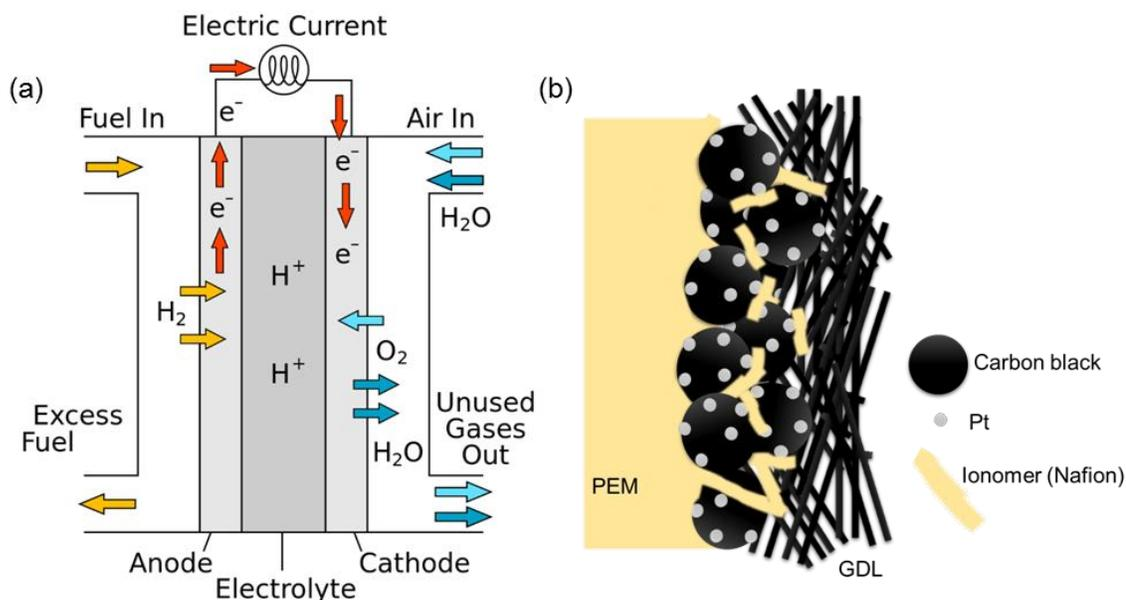
**Figure 1-1. Schematic of PEMFC operation (a) and a schematic of an electrode structure showing the catalyst layer between the PEM and GDL (b). The GDL represents a carbon fiber structure that is commonly used.**
