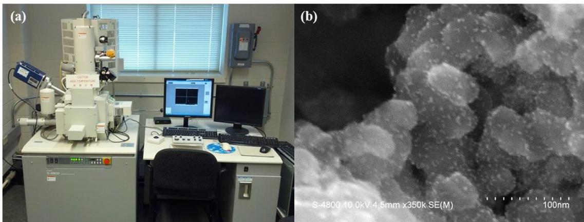
**Figure 2-3. (a) Photograph of Hitachi S-4800 SEM instrument at UWO. (b) Typical SEM image of Pt on carbon black catalyst using 10 kV acceleration voltage and mixed detectors in SE mode to enhanced the elemental contrast.**
