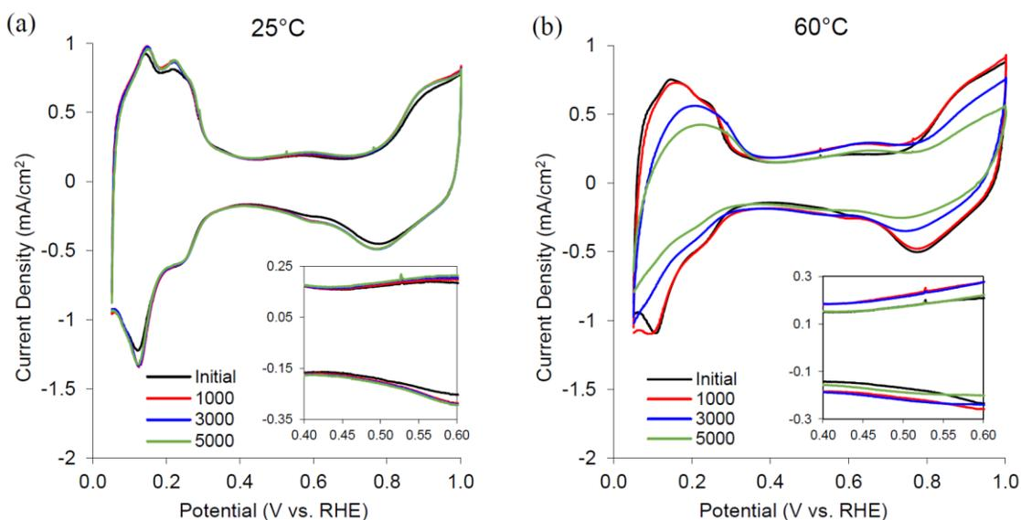
**Figure 5-3. Cyclic voltammograms of HSC catalyst at different cycles for (a) 25°C and (b) 60°C. Cycling at 500 mV/s from 1.0 – 1.5 V vs. RHE in 0.09 M H<sub>2</sub>SO<sub>4</sub>.**
