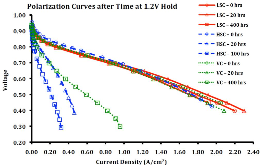
**Figure 5-1. Polarization curves for catalysts supported on LSC, VC, and HSC after different hold times at 1.2 V. Tests were carried out using a 50 cm<sup>2</sup> fuel cell with serpentine hardware, operated at 80°C in saturated H<sub>2</sub>/N<sub>2</sub> at 150 kPa absolute pressure for 400 hour**
