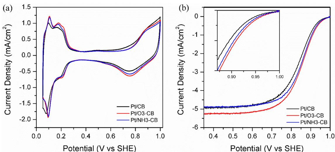
**Figure 4-5. CV curves normalized to Pt loading (a) and ORR polarization curves at rotation rate of 1600 RPM for Pt/CB, Pt/O<sub>3</sub>-CB, Pt/NH<sub>3</sub>-CB. Recorded in N<sub>2</sub> (a) and O<sub>2</sub> (b) saturated 0.5 M H<sub>2</sub>SO<sub>4</sub> with a scan rate of 20 mV/s.**
