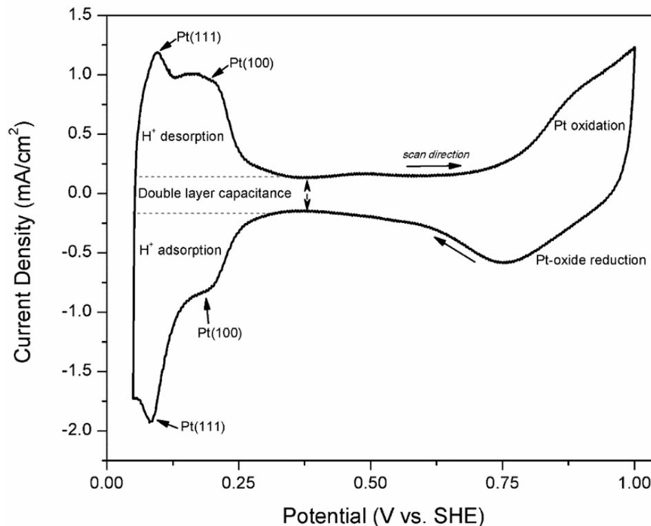
**Figure 1-4. A typical CV curve of a Pt/C catalyst in 0.5 M H<sub>2</sub>SO<sub>4</sub>. Labels indicating several regions of the curve where formation of electrochemical species creates easily identifiable peaks.**
