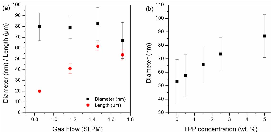
**Figure 3-2. (a) Average PNCNT diameter (in nm) and length (in  $\mu\text{m}$ ) for various Ar flow rates with precursor TPP concentration of 2.5 wt. %. (b) Average diameter of PNCNTs as a function of the TPP concentration in the precursor mixture, grown with 1.72 SLPM Ar flow.**
