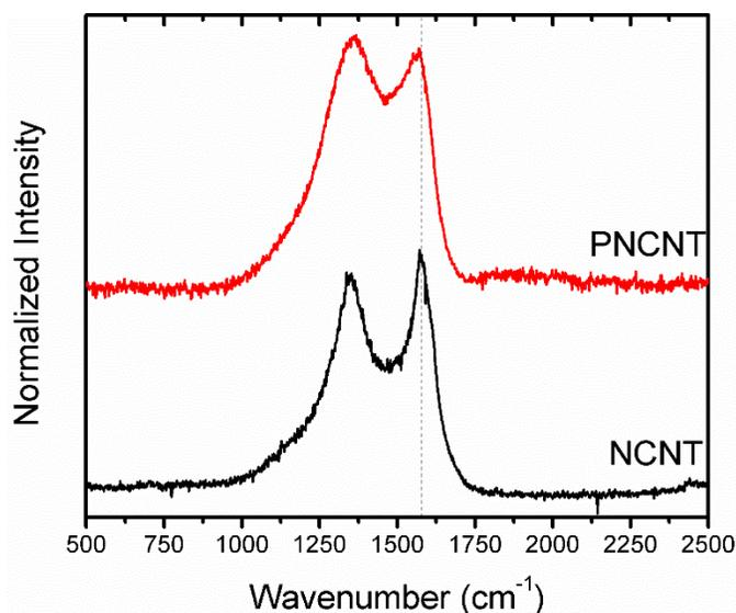
**Figure 3-4. Raman spectra of NCNTs and PNCNTs**
