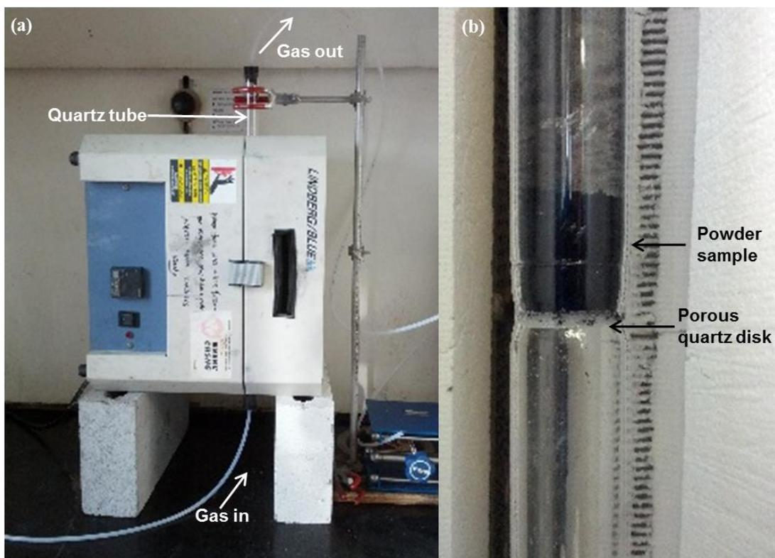
**Figure 2-2. Experimental setup for ammonia treatment of carbon nanomaterials. (a) Tube furnace with inlet and outlet gas lines visible at the bottom and top of the quartz tube. (b) Image of a carbon powder sample in the center of reaction tube, supported on a fritted quartz disk.**
