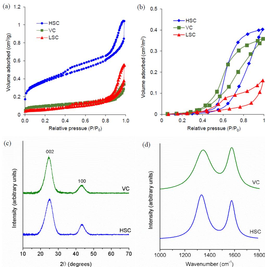
**Figure 5-2. (a) Sorption isotherms of H<sub>2</sub>O (a) and N<sub>2</sub> (b) on HSC, VC, and LSC (exclusive of Pt). (c) XRD and (d) Raman spectra of HSC and VC.**
