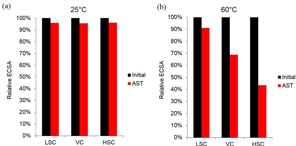
**Figure 5-4. Calculated ECSA at BOL and after 5000 cycles for catalysts on HSC, VC, and LSC at 25°C (a) and 60°C (b). 5000 cycles at 500 mV/s from 1.0 – 1.5 V vs. RHE in 0.09 M H<sub>2</sub>SO<sub>4</sub>.**
