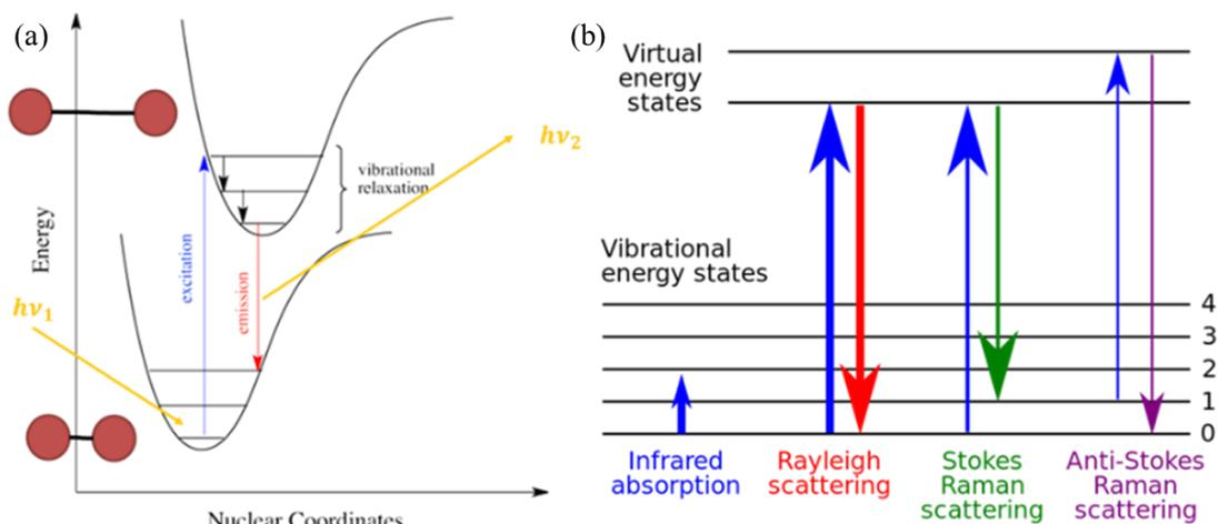
**Figure 2-6. (a) Molecular vibrational energy states of a molecule in high and low energy states, showing incident and emitted photons. (b) Photon absorption and emission energies for different scattering mechanisms.**
