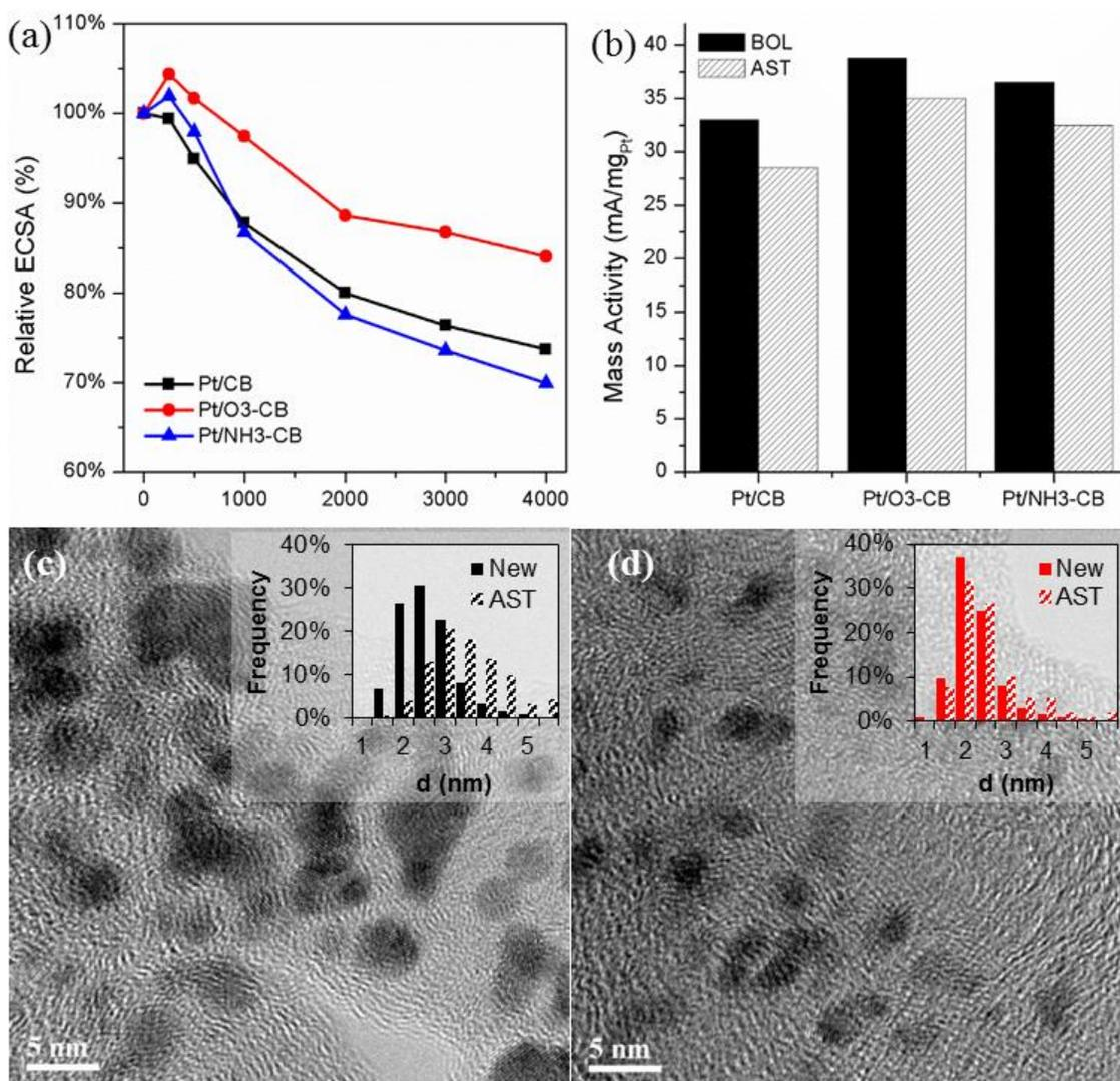
**Figure 4-6.** Relative ECSA values during AST cycling (a) and MA before and after AST (b) for Pt/CB, Pt/O<sub>3</sub>-CB, and Pt/NH<sub>3</sub>-CB. TEM images of Pt/CB (c) and Pt/O<sub>3</sub>-CB (d) after AST. The insets in (c) and (d) show histograms of the particle size distribution before and after AST. Cycling was done from 0.6-1.0 V in N<sub>2</sub> saturated 0.5 M H<sub>2</sub>SO<sub>4</sub> at room temperature.
