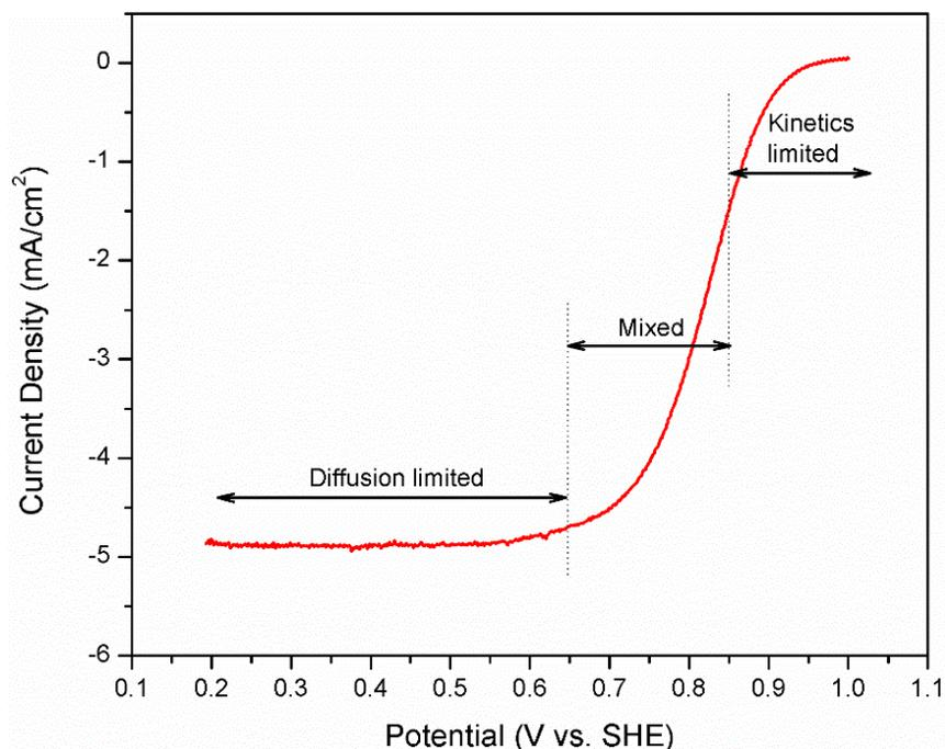
**Figure 1-5. ORR polarization curve of Pt/C catalyst recorded using RDE at 1600 RPM in O<sub>2</sub> saturated H<sub>2</sub>SO<sub>4</sub> at 25°C, scan rate 20 mV/s. The kinetic and diffusion limited regions are highlighted on the curve.**
