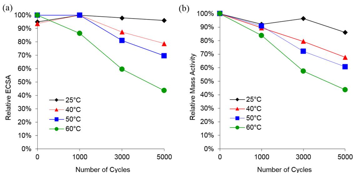
**Figure 5-5. ECSA (a) and mass activity (b) after AST cycling at 25, 40, 50, and 60°C for Pt/HSC. Cycling at 500 mV/s from 1.0 – 1.5 V vs. RHE in 0.09 M H<sub>2</sub>SO<sub>4</sub>.**
