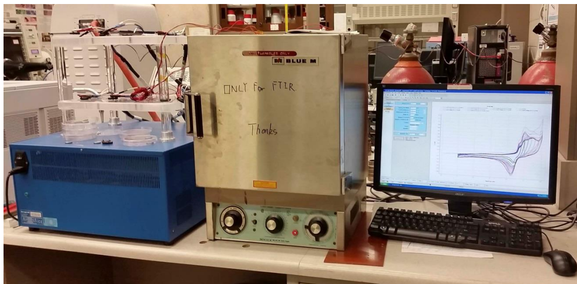
Figure 2.9. A photo of the VMP3 multichannel potentiostat 3/Z for CV and EIS measurements.
