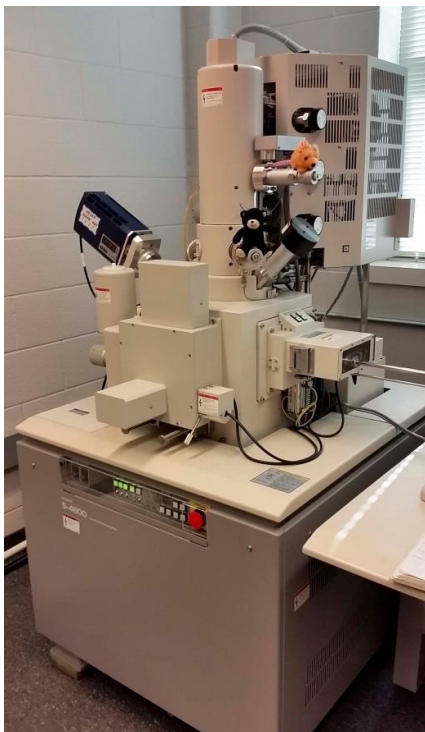
Figure 2.3. A photo of the Hitachi S-4800 field emission SEM equipped with and EDX spectrometer.
