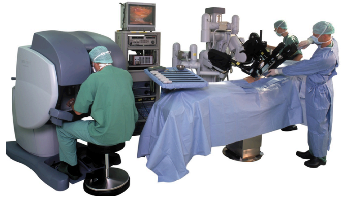
Figure. The da Vinci Surgical System. From left to right: surgeon console, vision system, patient-side cart and EndoWrist instruments. 9 Image ©[2013] Intuitive Surgical, Inc.
