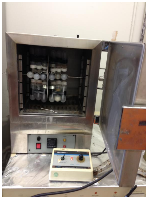
Figure S1. End over end shaker and oven used for batch experiments.
