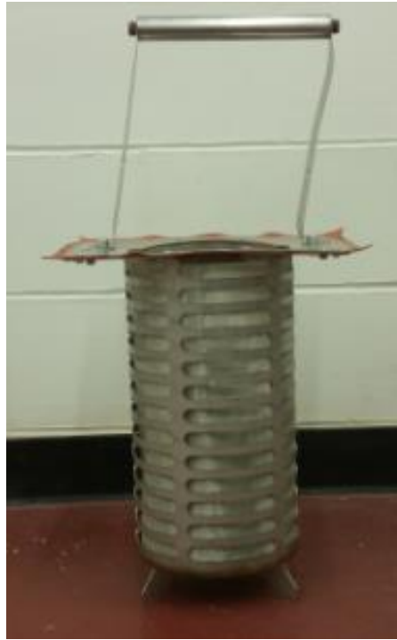
Figure 35: Sediment transport trap installed at the exit of the flume
