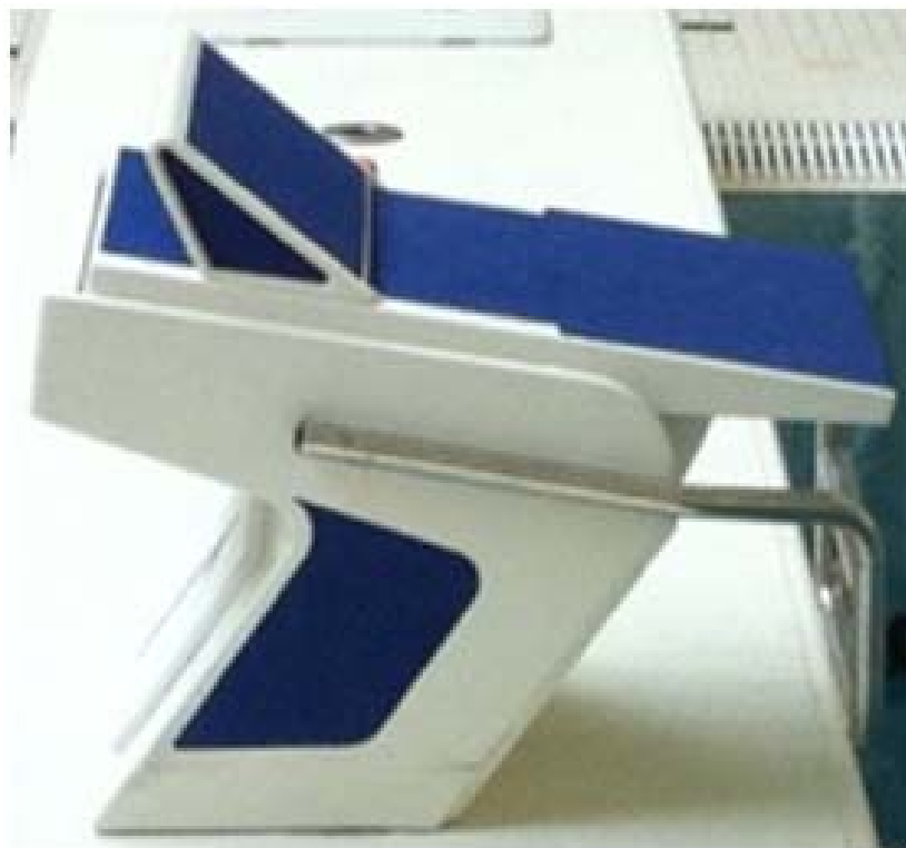
Figure 5.1: The Omega® OSB11 start block The kick plate is angled at 30 degrees from the surface of the platform. The platform is angled at nine degrees from horizontal.
