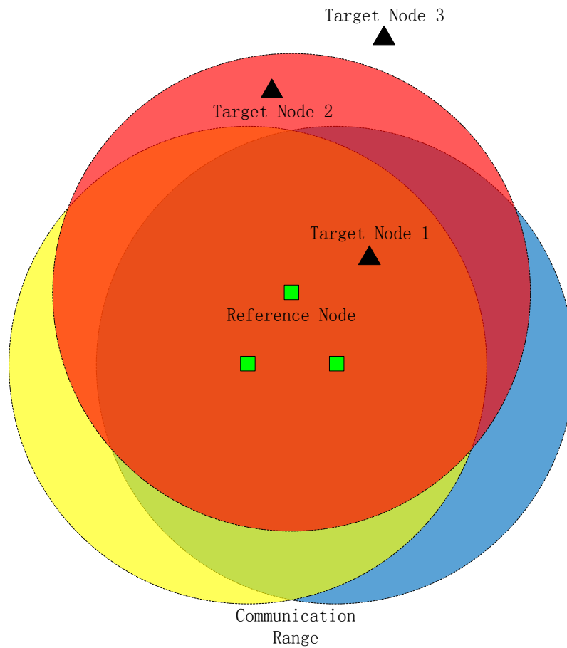
Figure 5.1: N selected reference nodes around the target
