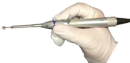
Figure 1.6: High speed rotary burring tool
