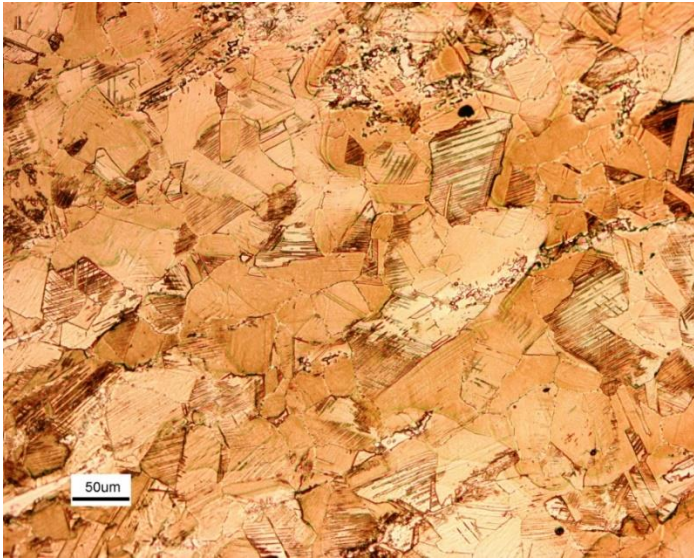
Figure 3.1 Microstructure of AISI 310 observed with an optical microscope.
