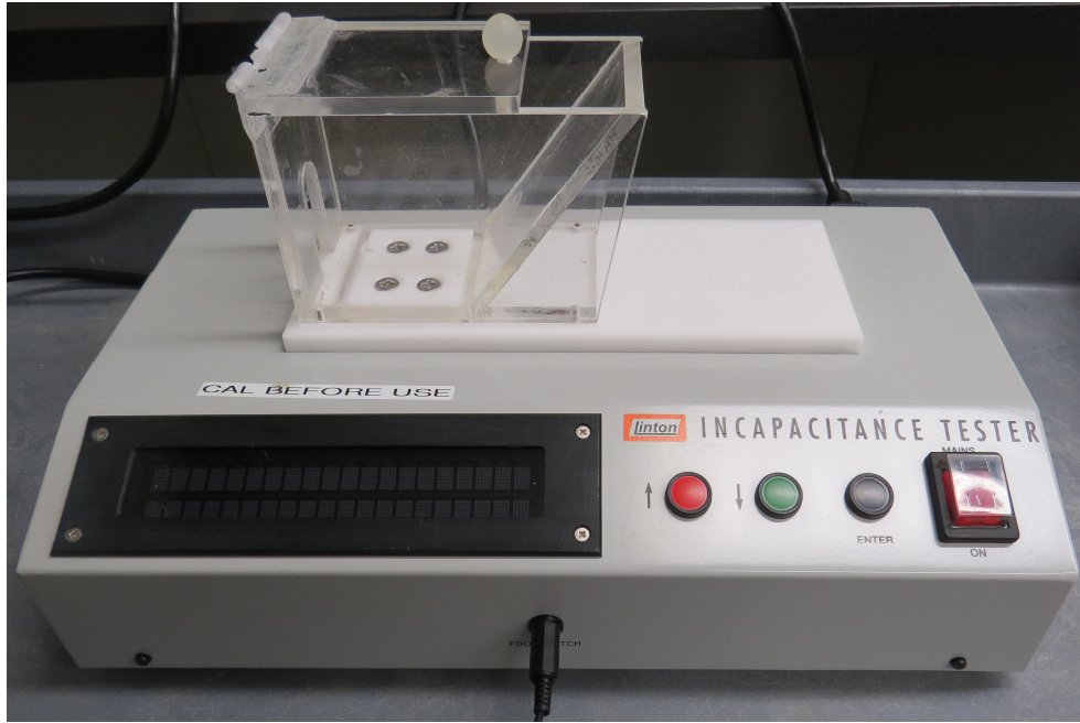
Figure 4.2: Incapacitance Tester. This instrument was used to assess static weight-bearing.
